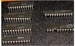
*Note the damage to the plastic on one chip.*
