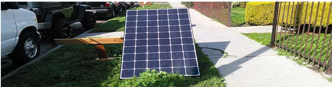
*Figure 1: The location and actual stand of the outside setup (only 1 of 2 panels mounted). The battery packs go under and behind the panels in a locked box fastened to the stand.*
