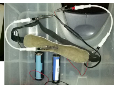
Figure 4: My equally errant eyeball warmer minus the electronics, shown fed by 2 batteries.
