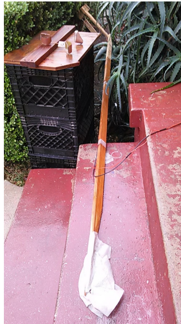
Figure 12: Upper part of broken mast
